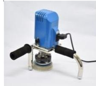
Design Intervention to ameliorate exposure to vibration during use of hand-held vibrating tools in unorganized sector (Stone-polishing work)
